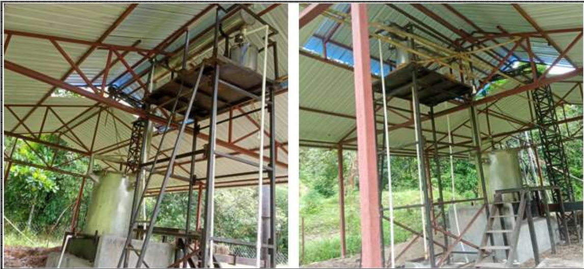
Cohabitation based Field Distillation Unit (Capacity 250 kg) at Kakoi village, Papumpare district, Arunachal Pradesh
